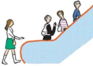
An escalator can operate continuously between specified days and times. It can also be set to conserve energy by operating outside those times only when a person approaches the escalator.
