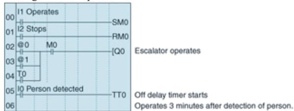
Use two weekly timers for the 7:00 to 10:00 and 17:00 to 22:00 weekday operation. For the rest of the time, use an OFF delay timer to operate the escalator for 3 minutes when pedestrians are detected.
