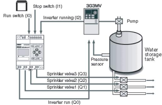
\*The 3G3MV has built-in PID function that allows the Inverter to control pressure inside the water storage tank.
