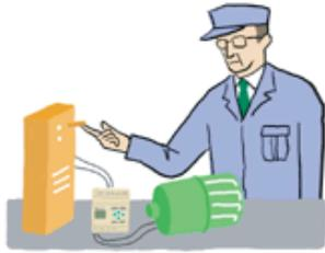
This application turns devices ON and OFF in tests, such as in durability tests. Pressing the run switch turns the device ON and OFF repeatedly for the preset amount of time. It stops automatically at the preset count.
