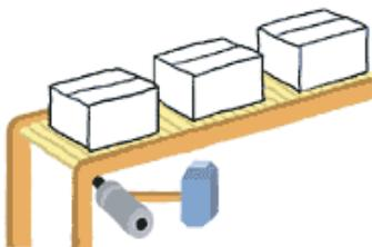
The inverter positions products of a specified distance.
