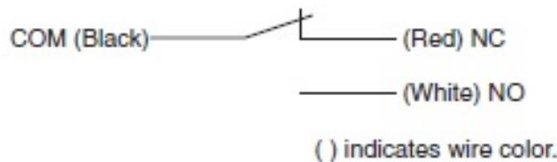
Note: The Z-15GM is a reversible model and the NO and NC positions are reversed.
