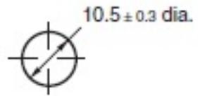
**Note: Recommended panel thickness: 1 to 4 mm.**
