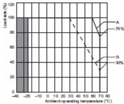
**Note:** 1. Multiply the above-shown load ratio by the coefficient of load reduction to input voltage.
