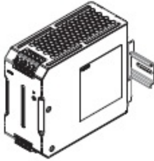
(A) Standard (Vertical) mounting
