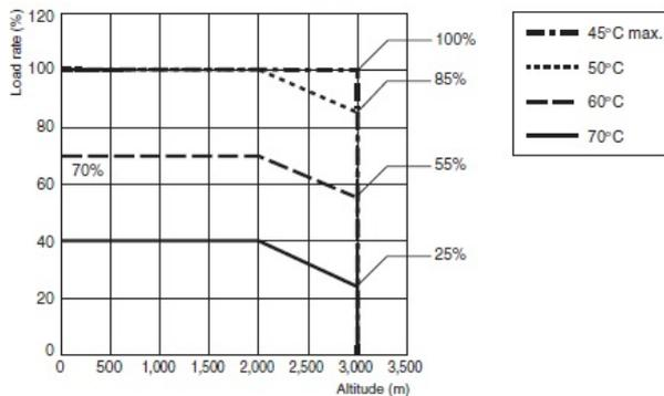
**Note:** At a voltage below 100 VAC, reduce the load at the rate of 1.3%/V. (40°C < Ambient temperature ≤ 70°C)
