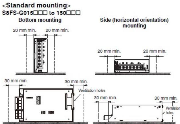
**Note:** Use a metal plate as the mounting surface.
