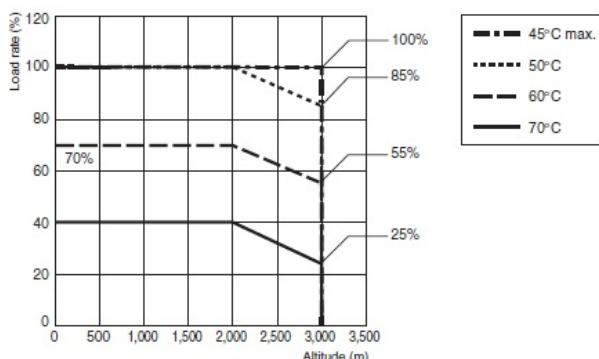
**Note:** At a voltage below 100 VAC, reduce the load at the rate of 1.3%/V. ( $40^{\circ}\text{C} < \text{Ambient temperature} \leq 70^{\circ}\text{C}$ )
