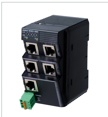
Industrial Switching Hub W4S1-05D
