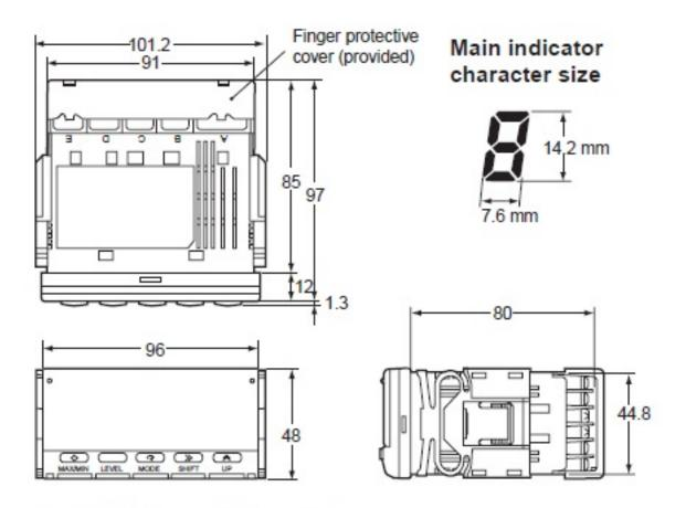
The K3MA-L uses M3 terminals. A terminal cover is provided.
