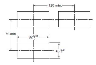
Mounting Recommended Panel Thickness 1 to 8 mm. Mount the product horizontally.
