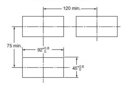
Mounting Recommended Panel Thickness 1 to 8 mm.
