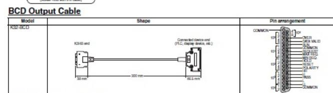
Note: The BCD Output Cable has a D-sub plug.
