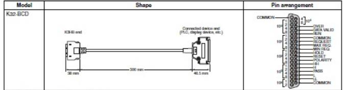
Note: The BCD Output Cable has a D-sub plug.
