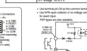
Note: A 3-wire DC sensor can also be connected. Check the ratings and characteristics table, however, for the connection conditions.
