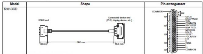
**Special Cable (for Event Inputs with 8-pin Connector)**
