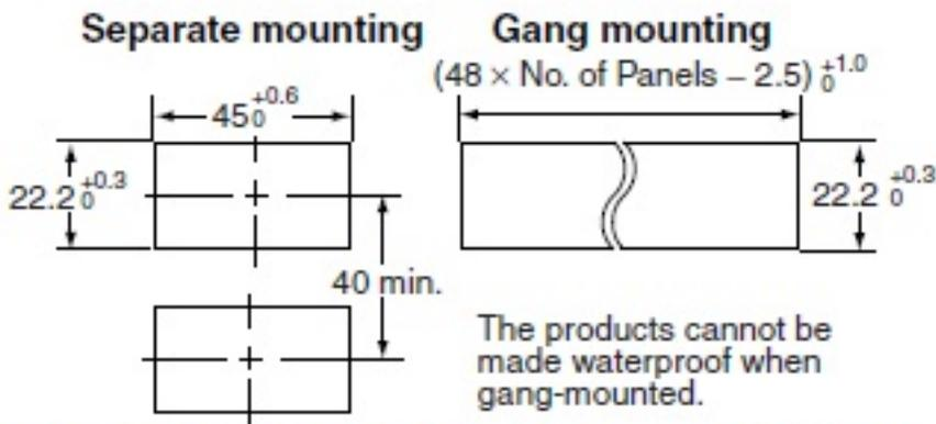
Mounting Recommended Panel Thickness 1 to 5 mm.
