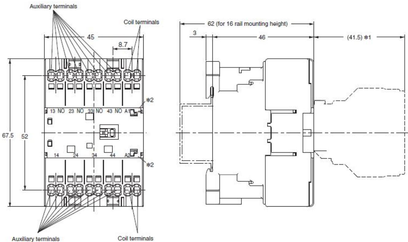
\*1. When auxiliary contact unit (J73KC) is mounted
