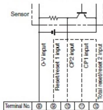
**Note:** When using the H7BX as a tachometer, do not use the CP2 input or total reset/reset 2 input.
