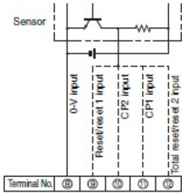
Operates when the transistor turns OFF.
