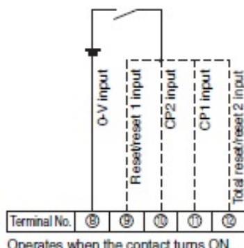
Operates when the contact turns ON.
