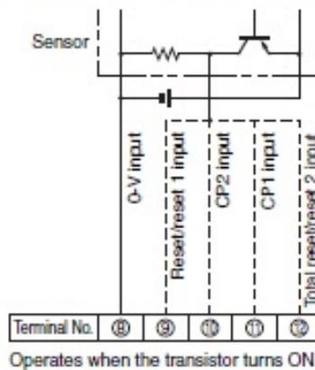
**Note:** When using the H7BX as a tachometer, do not use the CP2 input or total reset/reset 2 input.
