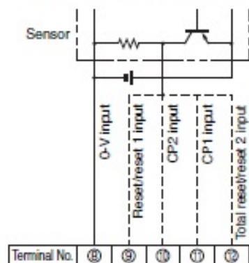
Operates when the transistor turns ON.
