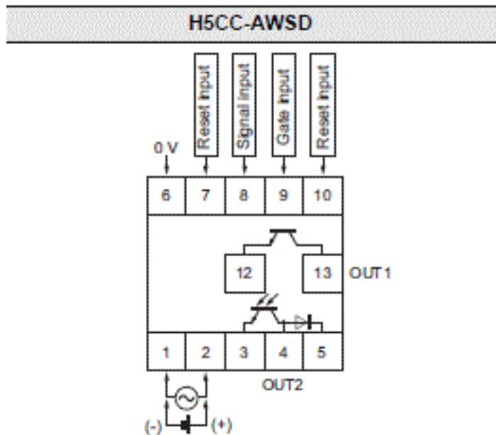
**Note:** Terminals 7 and 10 have the same reset function. The same function will be performed whichever terminal is connected. Terminals 7 and 10 are not connected internally, however, so do not use them for cross-over wiring.
