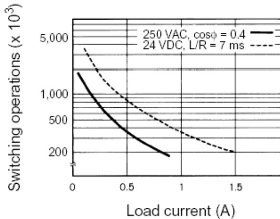
Reference: A maximum current of 0.5 A can be switched at 125 VDC ( $\cos\phi = 1$ ).
