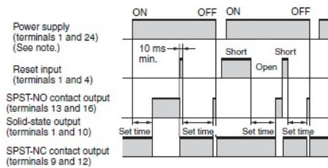
**Note:** When using a 12/24 V DC-operated model with a 12 V DC power supply, short terminals 13 and 15.
