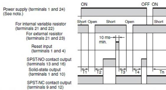
**Note:** 1. Control output is provided when the set time has elapsed ( $T_1 + T_2$  or  $T_3 + T_4$ ).
