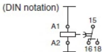
**Note:** The above figure shows the terminal arrangement for a 24 to 48-VAC/DC model. Models with 100 to 120-VAC or 200 to 240-VAC power input do not have a DC input.
