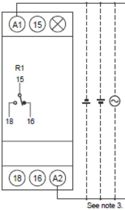
**Note 3: The power supply terminals do not have polarity.**
