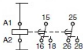
Note: The power supply terminals do not have polarity.
