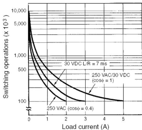
Reference: A maximum current of 0.15 A can be switched at 125 VDC ( $\cos\phi = 1$ ) and a maximum current of 0.1 A can be switched if L/R is 7 ms. In both cases, a life of 100,000 operations can be expected. The minimum applicable load is 10 mA (100 mA for H3CR-A8E) at 5 VDC (failure level: P).
