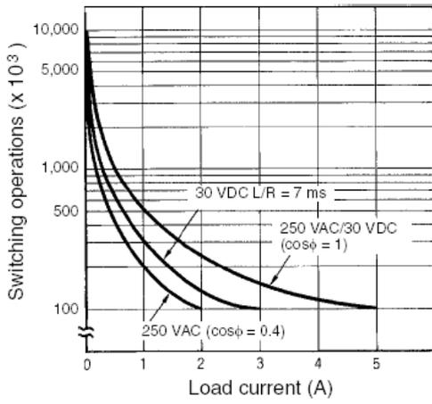
Reference: A maximum current of 0.15 A can be switched at 125 VDC ( $\cos\phi = 1$ ) and a maximum current of 0.1 A can be switched if L/R is 7 ms. In both cases, a life of 100,000 operations can be expected. The minimum applicable load is 10 mA (100 mA for H3CR-A8E) at 5 VDC (failure level: P).
