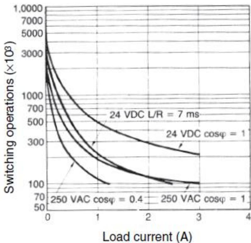
Reference: A maximum current of 0.15 A can be switched at 125 VDC ( $\cos\phi = 1$ ). Maximum current of 0.1 A can be switched if  $L/R$  is 7 ms. In both cases, a life of 100,000 operations can be expected.
