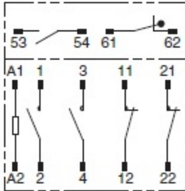
**Note:** The coil has no polarity.
