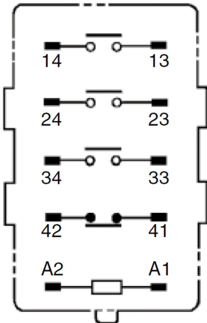
The coil has no polarity.
