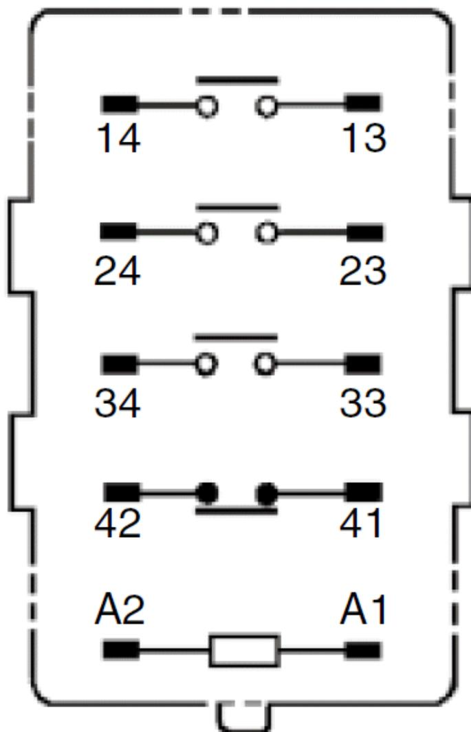
The coil has no polarity.
