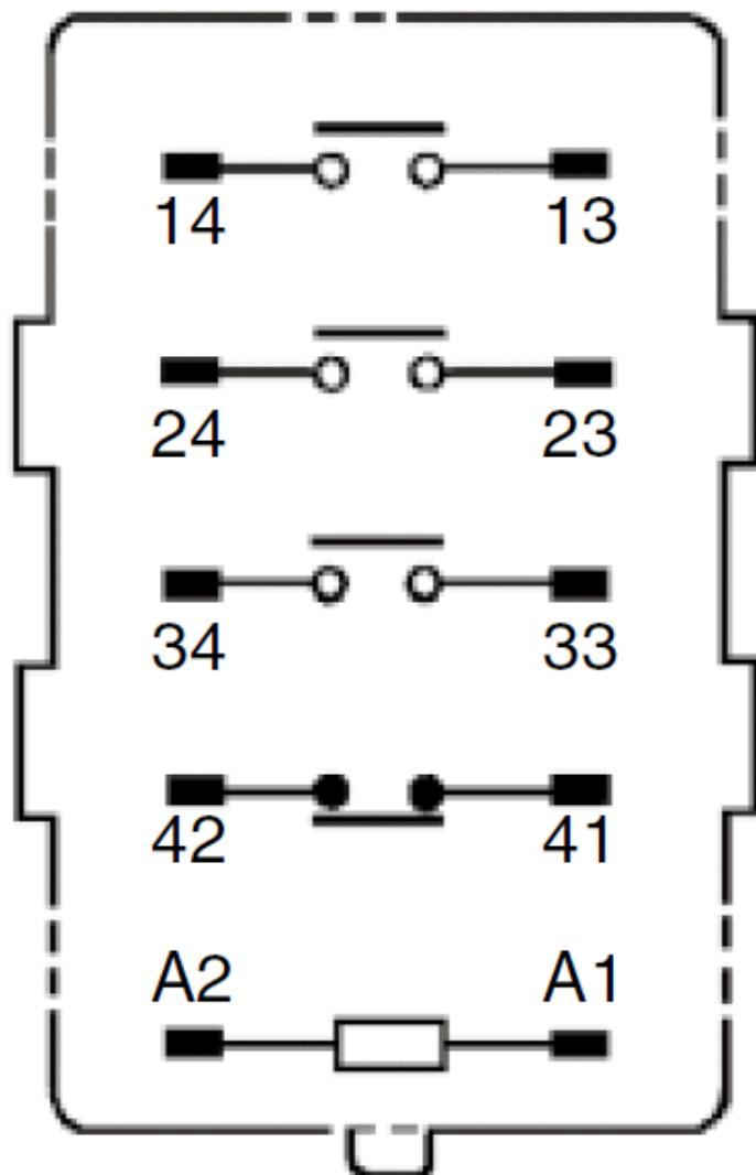
The coil has no polarity.
