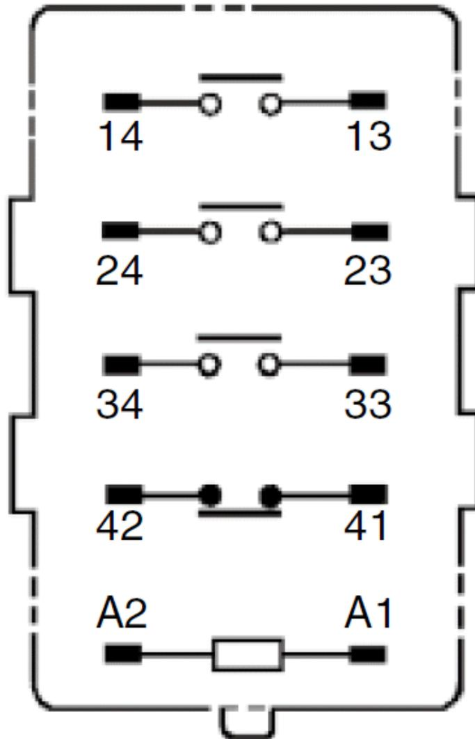
The coil has no polarity.
