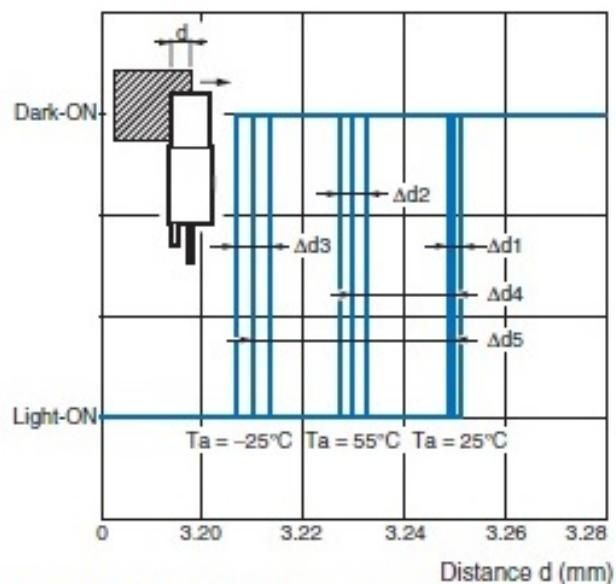
$V_{cc} = 12\text{ V}$ , No. of repetitions: 20,  $\Delta d_1 = 0.002\text{ mm}$ ,
