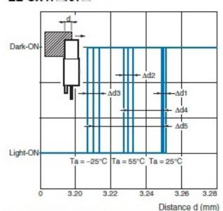
Vcc =12 V, No. of repetitions: 20, Δd1 = 0.002 mm,  $\Delta d2 = 0.004 \text{ mm}, \ \Delta d3 = 0.005 \text{ mm}, \ \Delta d4 = 0.02 \text{ mm},$
