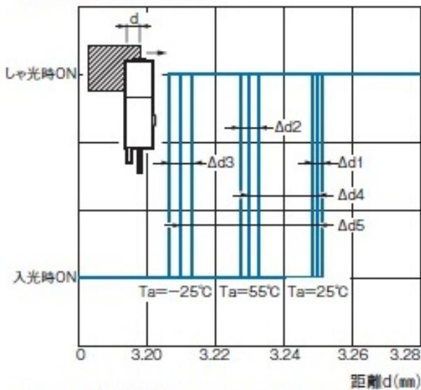
$V_{CC}=12V$  繰返し数: 20  $\Delta d1=0.002mm$   $\Delta d2=0.004mm$   $\Delta d3=0.005mm$   $\Delta d4=0.02mm$   $\Delta d5=0.04mm$
