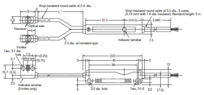
\*L = 500 mm (EE-SPW321, EE-SPW421) L = 1,000 mm (EE-SPW321-A, EE-SPW421-A)
