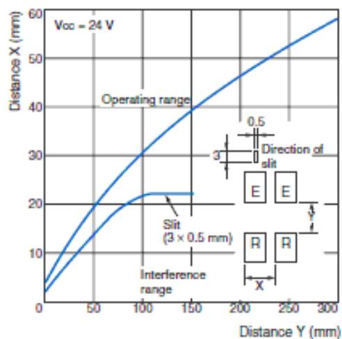
**Sensing Distance vs. Input Voltage**
