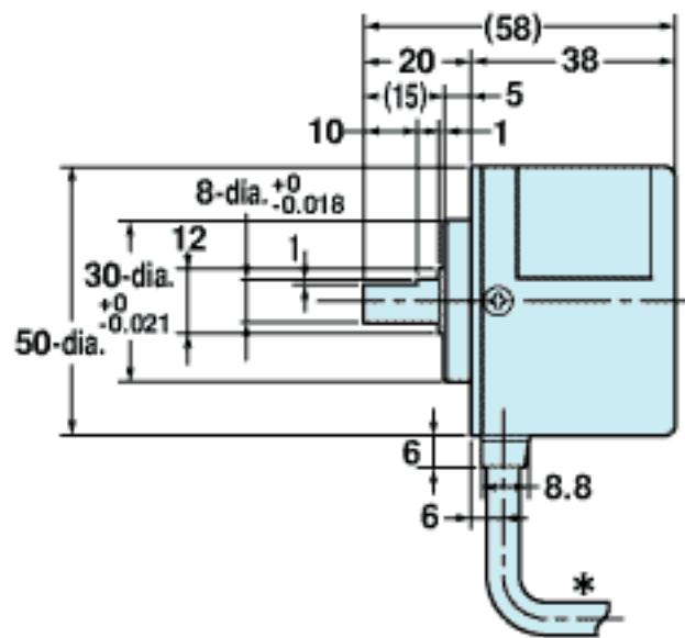
\* 6-dia. Oil-resistant PVC-insulated shielded cable with 12 conductors
