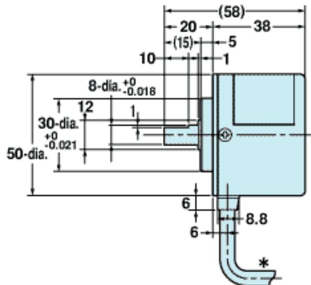
\*6-dia. Oil-resistant PVC-insulated shielded cable with 12 conductors
