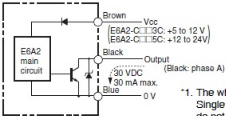
\*1. The white and orange wires of Single Models (E6A2-CS□□) do not output signals (no connection).
