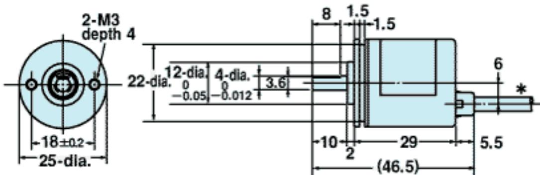
\* 4-dia. Vinyl-insulated round cable with 5 conductors
