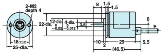
\*4-dia. Vinyl-insulated round cable with 5 conductors (conductor cross section: 0.14mm², insulator diameter: 0.9mm) Standard length: 500mm
