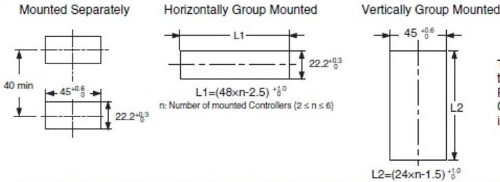
To mount the Temperature Controller so that it is waterproof, insert the Waterproof Packing onto the Temperature Controller. Group mounting does not allow waterproofing.
