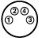
M8 Connector Pin Arrangement
