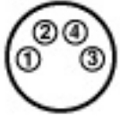
M8 Connector Pin Arrangement
