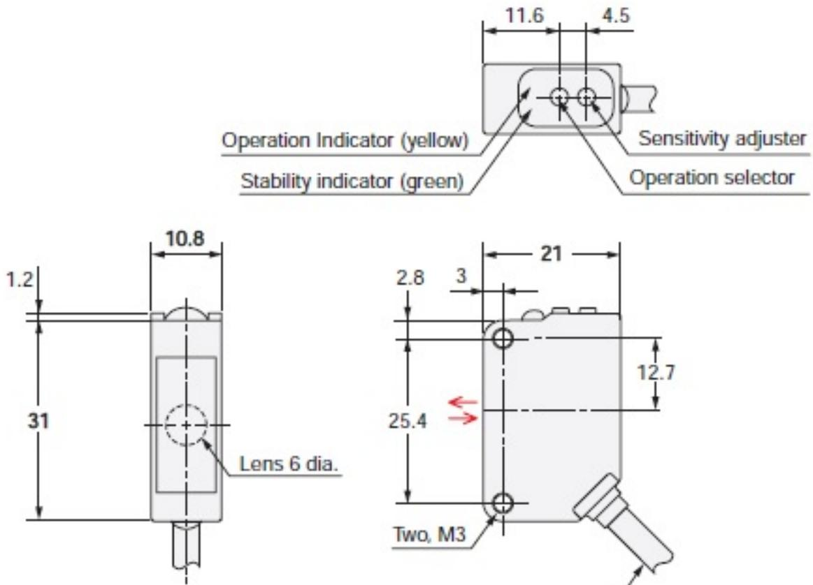
4 dia. vinyl-insulated round cable with 3 conductors (Conductor cross section:0.2 mm<sup>2</sup> (AWG24), Insulator diameter:1.1 mm), Standard length: 2 m
