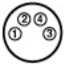
M8 Connector Pin Arrangement
