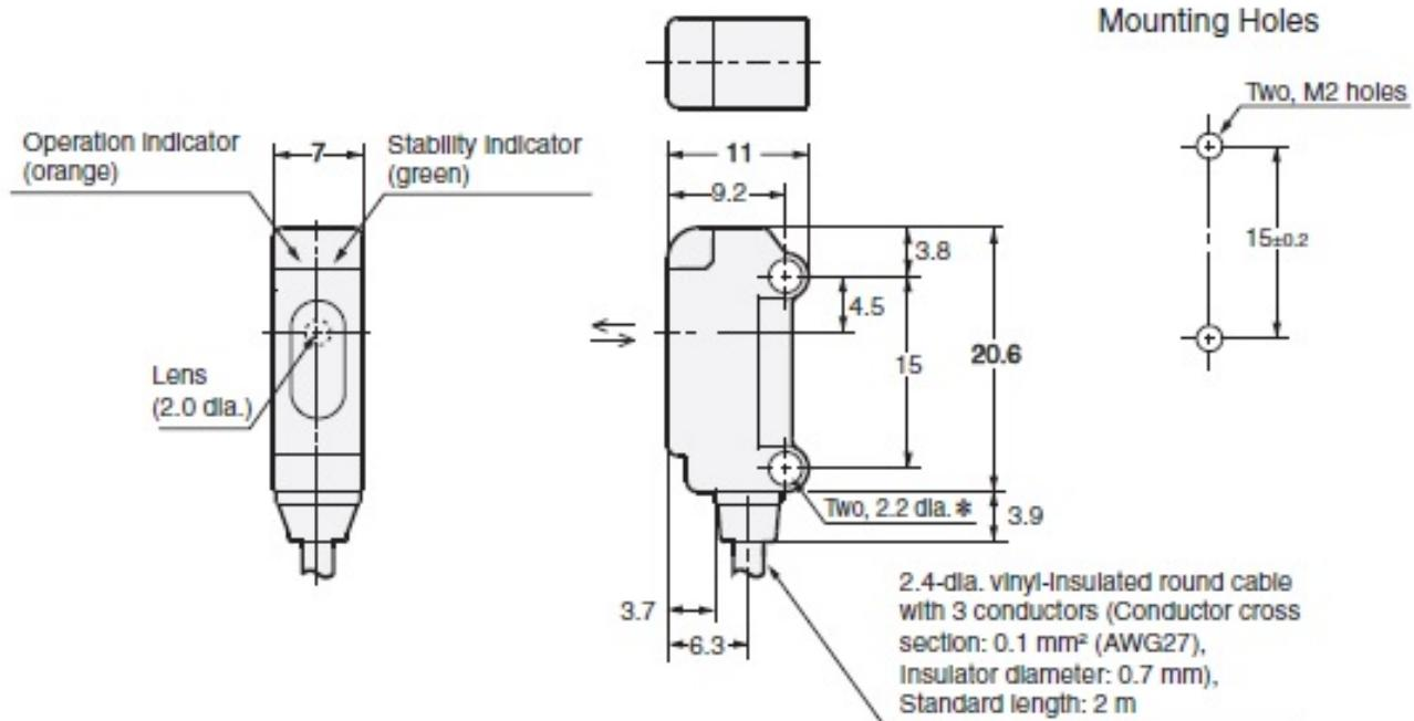
\*The mounting holes are made of SUS301.
