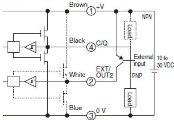
Using Pin 2 with a control output
