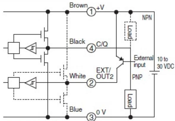
Using Pin 2 with a control output
