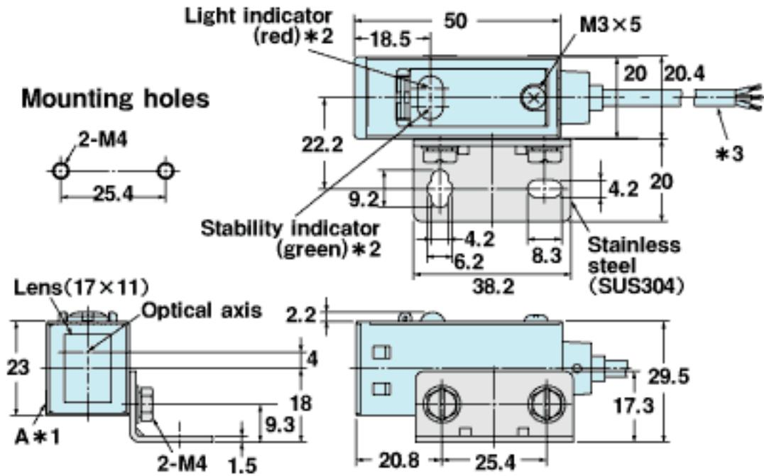
\*1. The mounting bracket can be attached to side A.
