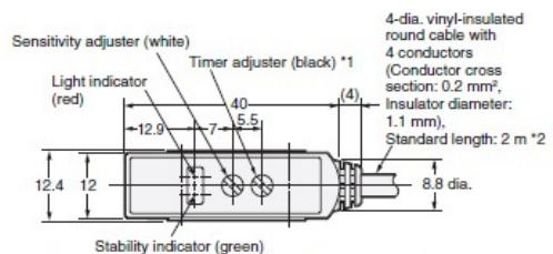
\*1. Not applicable to Sensors with timer adjusters (E3S-AT11 and E3S-AT31).
