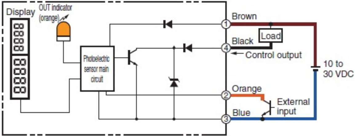
Note: 1, 2, 3 and 4 are pin terminals of M8 Connector Type.
