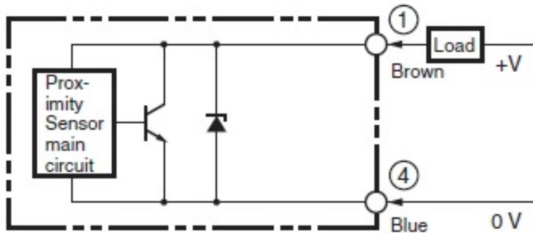
Connector Pin Arrangement
